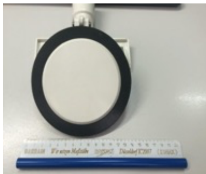
FIGURE 2 REFLUX VALVE FLAP AND SEAL
